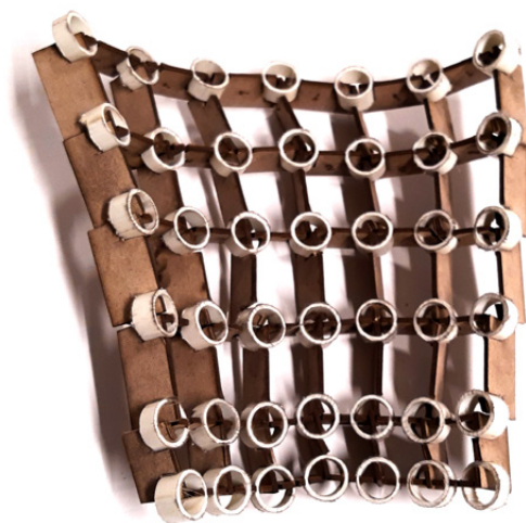
FIGURE 18: Singly Curved assembled Fixed-Joint Shell
