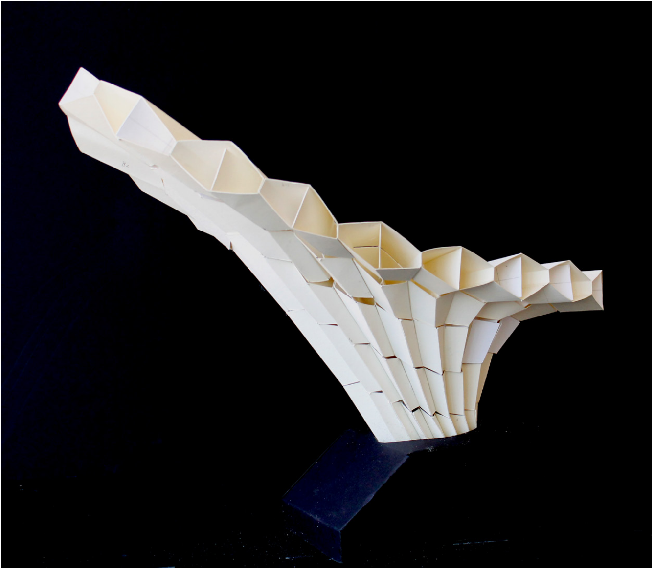
FIGURE 34: 1:100 Scale prototype: Polygonal modules with plug-type joints
