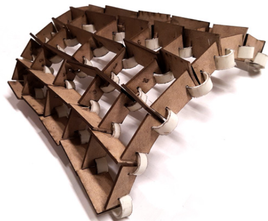
FIGURE 19: Singly Curved assembled Fixed-Joint Shell
