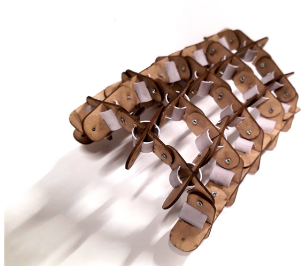
FIGURE 17: Singly Curved Hinged-Joint Shell
